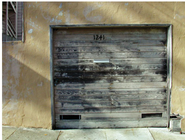
FIGURE 4.9 Wide-angle lenses often suffer from a bit of barrel distortion. Although it's slight in this image, you can see it along the top of the garage door.
